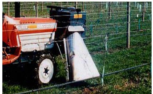
Figure 11. Trialing vineyard weed control with super-heated steam from a new Vaporjet® thermal weeder.
