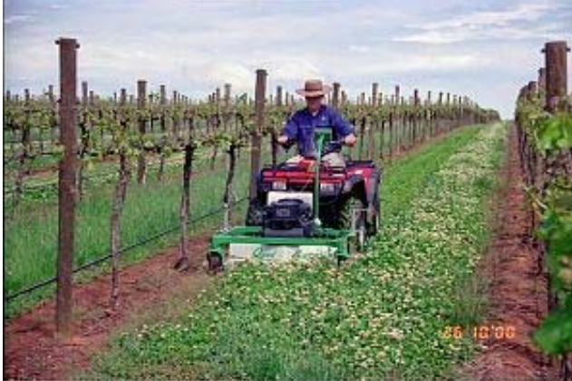
Figure 9. Lighter alternatives to tractor-driven mowers can be used to reduce vineyard soil compaction.
