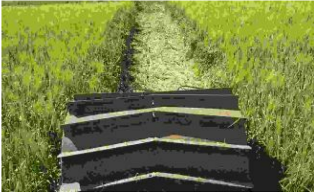
Figure 12. The ribbed roller shows promise for vineyard weed management.
